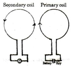
$\phi \propto i \Rightarrow \phi = Mi$ .....(1) for N turns,  $N\phi = Mi$
