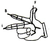
Stretch fore-finger, central finger and thumb of right hand mutually perpendicular to each other. If fore-finger represents the direction of magnetic field, the thumb represents the direction of motion of the conductor, and then the central finger indicates the direction of induced current.
