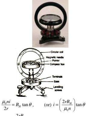
Where  $\frac{2rB_H}{\mu_o n}$  is called reduction factor (K)of tangent galvanometer.  $\therefore i = K \tan \theta$
