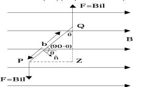
If the coil consists of 'N' turns,  $\tau = BiAN \sin \theta$ In vectorial form,  $\vec{\tau} = Ni(\vec{A} \times \vec{B})$
