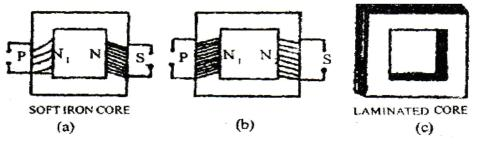
If  $N_1$  and  $N_2$  be number of turns in primary & secondary coils  $E_1$  and  $E_2$  be induced e.m.f. in primary and secondary coils, we have
