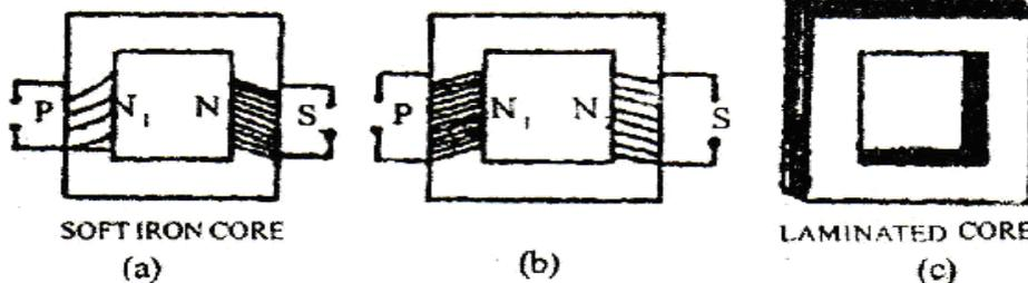
If  $N_1$  and  $N_2$  be number of turns in primary & secondary coils  $E_1$  and  $E_2$  be induced e.m.f. in primary and secondary coils, we have
