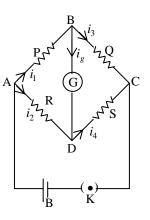
When the key K is pressed, Let  $i_1, i_2, i_3$  and  $i_4$  be the currents
