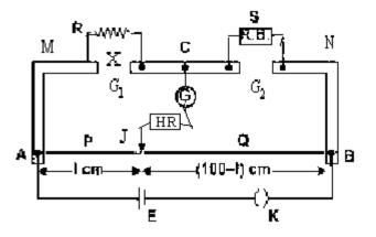
**Measurement of unknown resistance :** A battery of emf E is connected between A and B through a plug key K. An unknown resistance X is connected in the left gap  $G_1$  and a resistance box R.B. is connected in the right gap. A high resistance HR and a galvanometer G and a Jockey J are connected in series to central terminal C as shown. **Procedure :** A suitable resistance R is introduced in the R.B and the plug key K is
