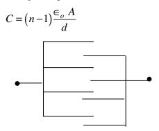
These capacitors are used in high frequency oscillating circuits. The dielectric constant of mica does not change with temperature and hence these capacitors are used as standard capacitors in laboratory.
