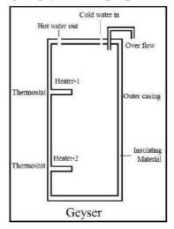
**Working of Geyser:** - 1. Geyser is an electrical device which converts the electrical energy into heat energy.
