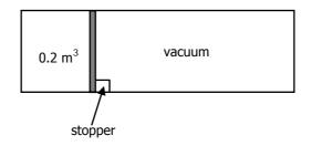
At certain instant of time t, the stopper is removed and the piston moves out freely to the other end. The final temperature is (*F*
