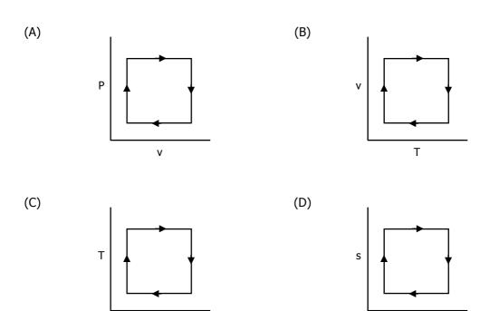
33. 2 kg of steam in a piston-cylinder device at 400 kPa and 175 °C undergoes a mechanically reversible, isothermal compression to a final pressure such that the steam becomes just saturated. What is the work, W, required for the process. Data:
