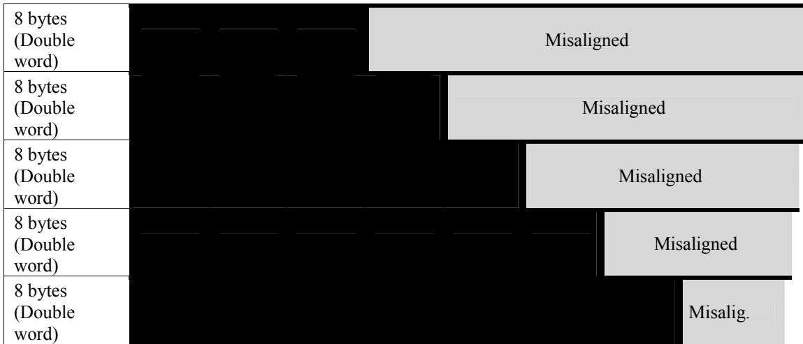
FIGURE 2.5 Aligned and misaligned addresses of byte, half word, word, and double word objects for byte addressed computers.
