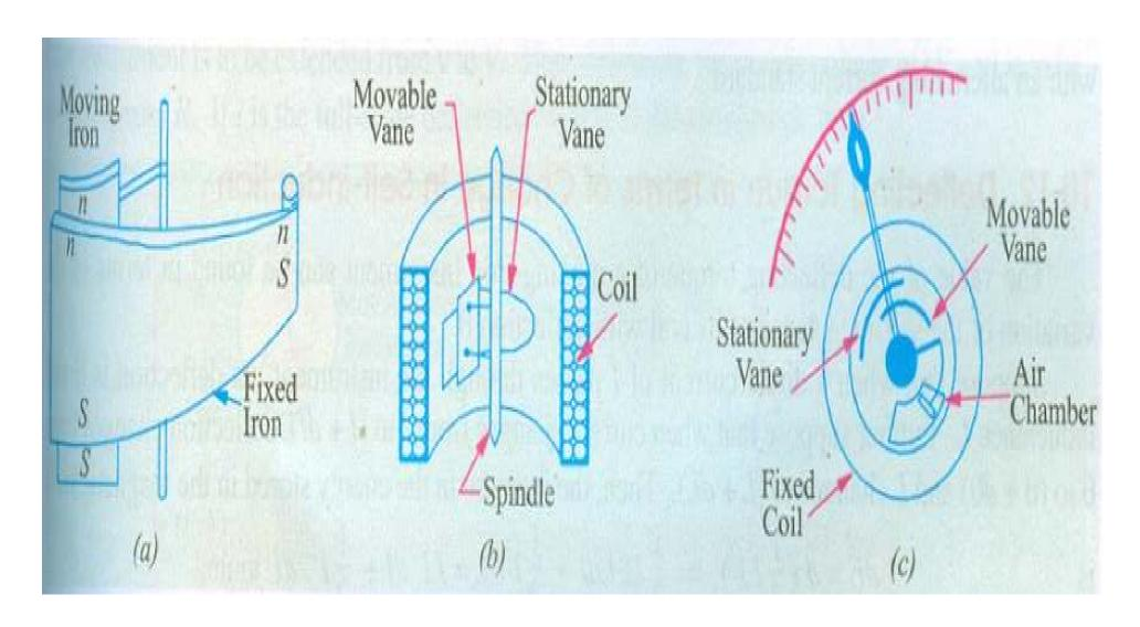
The deflecting torque is due to the repulsive force between the two similarly magnetised iron rods or sheets.
