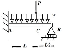
7. Using displacement method, derive the expressions for the stresses displacements of the body as shown below
