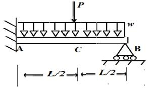
7. Using displacement method, derive the expressions for the stresses displacements of the steel beam with uniform cross section 'A' and lengths  $AC = L_1$  and  $CB = L_2$  as shown below
